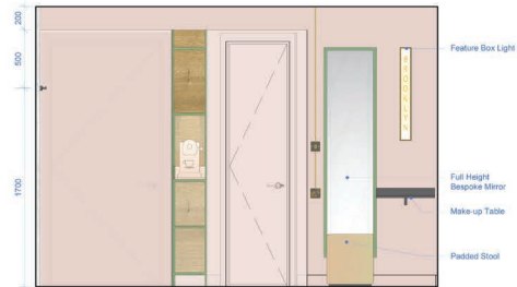
2 214 Bedroom Elevation- Room R214 Scale 1:25 @ A1
